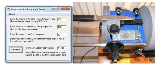
The same knives were then re-sharpened on Tormek-compatible 254 mm CBN wheels, and honed on a dedicated Tormek leather wheel impregnated with 3-micron diamonds. Edge bevel was ground on a CBN wheel #400, and edge set on a CBN wheel #1000. For honing on Tormek with diamonds we normally use a rock-hard felt wheel, but this time used the leather wheel to hone the same way as in the first sharpening.
