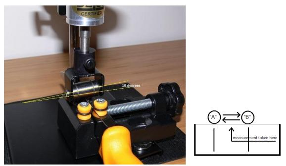
The impact roller is lowered at "A", then moved (rolled) over to "B" and then back to "A". A-B-A is one cycle.
