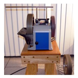
To match sharpening done with aluminium oxide and CBN/diamond, in each sharpening we set the edge with 2 passes on the #1000 aluminium oxide or CBN wheel, and were giving the edge the same amount of honing of 2-3 slow passes across the leather wheel, alternating sides.
