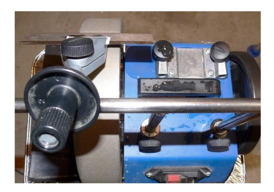
Deburring was done edge-trailing on a paper wheel with 5 micron diamonds at the exact edge angle, i.e. 15 dps, with the help of our <u>support for controlled-angle honing</u> and computer software. Finished on a paper wheel with 0.5 micron diamonds to see effect of burnishing.
