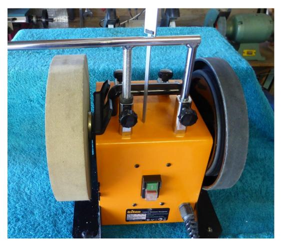
When we sharpen a batch of knives at the same angle, and keep the distance between the jig adjustable stop and the knife edge constant as we clamp new knives, we have to recalculate the Support height for a given grinding wheel only after truing that wheel. If for whatever reason we change the clamping distance, or have to sharpen at a different angle, we recalculate the Support height.
