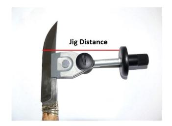
Run the application, enter the wheel diameter, jig distance, the target grinding angle in degrees per side, and press the Calculate button.
