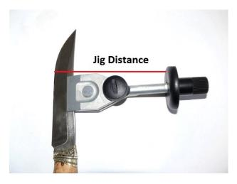
Run the application, enter the wheel diameter, jig distance and the target grinding angle in degrees per side, and press the Calculate button.
