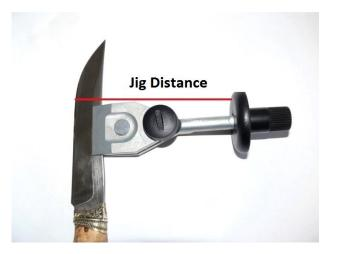
Run the application, select the grinding/honing option, enter the wheel diameter, jig distance and the target grinding angle in degrees per side, and press the Calculate button.
