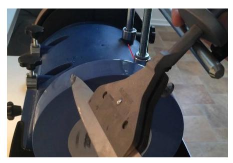
The Support bar height is set with the help of a caliper depth probe as shown below; position the depth probe parallel to the support legs, and perpendicular to the support horizontal bar.
