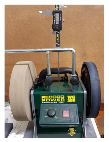
When we sharpen a batch of knives at the same angle, and keep the distance between the jig adjustable stop and the knife edge constant as we clamp new knives, we have to recalculate the Support height for a given grinding wheel only after truing that wheel. If for whatever reason we change the clamping distance, or have to sharpen at a different angle, we recalculate the Support height.
