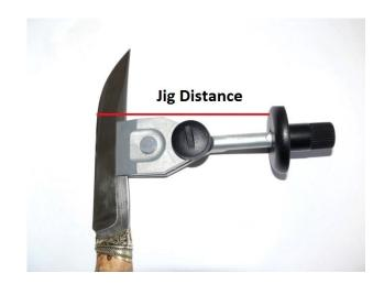
Run the application, select your model, enter the wheel diameter, jig distance, the target grinding angle in degrees per side, and press the Calculate button.
