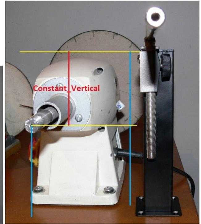
See how we measure the Constant\_Horizontal and Constant\_Vertical; must be done for each side, because distances are not the same on the left and right even in the best buffer/grinder.
