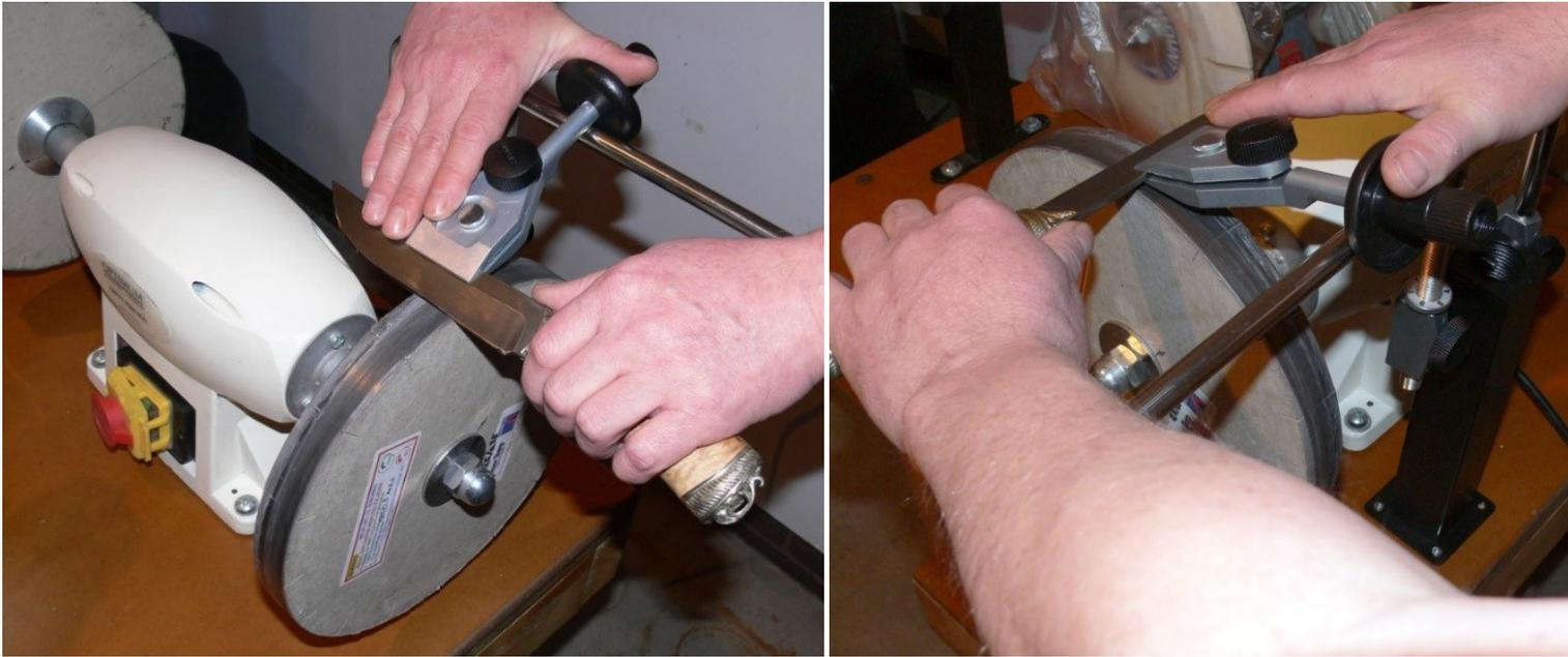
Move the knife over the paper wheel with light pressure just enough to maintain continuous contact of the blade with the wheel. Ensure that the blade is in contact with the entire width of the paper wheel; near the tip raise the knife handle following the taper. Half-speed buffer/grinder is recommended.
