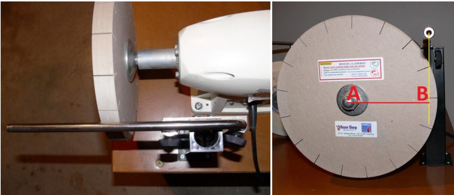
The distance **AB** between the grinder shaft centerline and the bar centerline should be approx. 9 cm for 8" paper wheel, and **12.5 cm for 10" paper wheel**. While parallel alignment of the grinder shaft and the support bar is very important, the distance AB can be approximate at this step.
