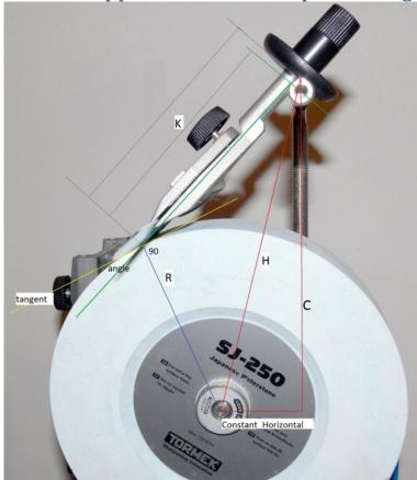
We use computer software to set a desired grinding angle. Time-wise it is quicker than any other method.
