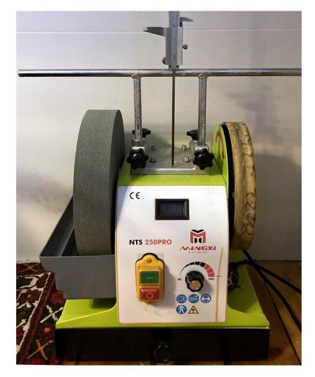
When we sharpen a batch of knives at the same angle, and keep the distance between the jig adjustable stop and the knife edge constant as we clamp new knives, we have to recalculate the Support height for a given grinding wheel only after truing that wheel.
