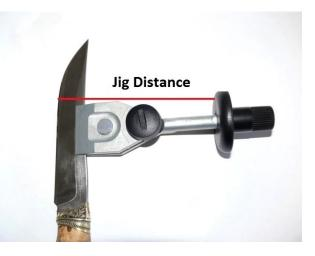
Run the application, enter the wheel diameter, jig distance and the target grinding angle in degrees per side, and press the Calculate button.
