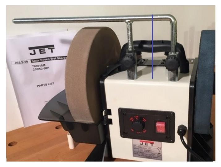
When we sharpen a batch of knives at the same angle, and keep the distance between the jig adjustable stop and the knife edge constant as we clamp new knives, we have to recalculate the Support height for a given grinding wheel only after truing that wheel. If for whatever reason we change the clamping distance, or have to sharpen at a different angle, we recalculate the Support height.
