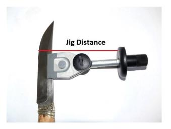
Run the application, enter the wheel diameter, jig distance and the target grinding angle in degrees per side, and press the Calculate button.
