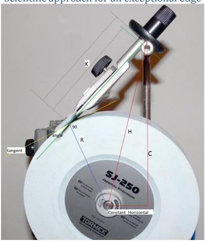
We use computer software to set a desired grinding angle with 0.1 degree accuracy.
