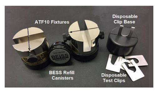
When cutting or severing a material, we all know that a dull edge will require more applied force than a sharp edge to accomplish the same task. It is this well-known and simple premise that EOU has used as a design basis for our edge testers. Less force = a sharper edge and more force = a duller edge. It's a simple instrumentation recipe and that has only two main ingredients: (1) an accurate instrument capable of recording and calculating the maximum test force
