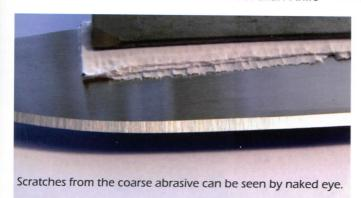
When I am happy with the bevels I've created, I set edge on a #1000 grit CBN wheel. Again, using computer software to maintain the same angle we shaped the bevels. This method gives us a razor edge even at this stage. When I say razor, I mean true razor edge, not just shaving!
