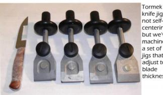
knife jig is not selfcentering, but we've machined a set of jigs that adjust to blade thickness.
