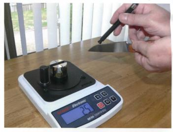
samples only one point on the edge, even when you take a couple of measurements at points of the blade. At Knife Grinders we check edge by two devices used together: a BESS PT50 edge sharpness tester and the Razor-Edge edge tester.
